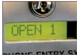
built-in display indicates door/gate has been opened
