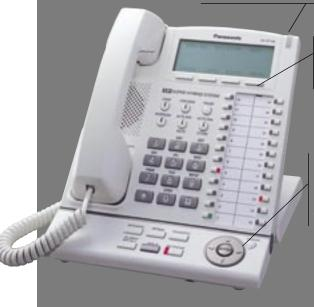
Soft keys are used in display to select a function.
